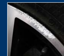
Curb scuff repair*
